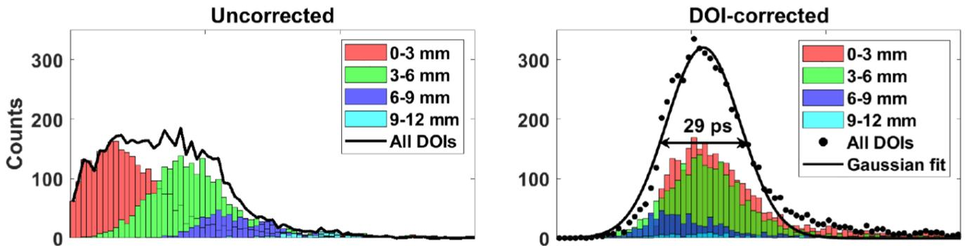
Figure 1: Example of a (left) non corrected and (right) DOI-corrected Cherenkov photons' detection time distribution.
